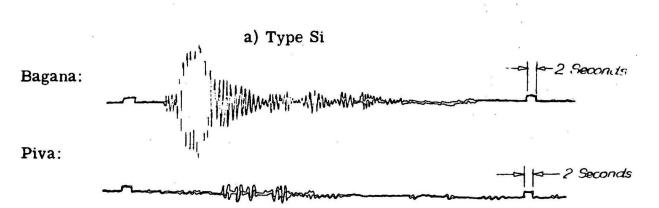
Bagana: strong impulsive first movement; ground motion indifferently up or down; duration more than 40 sec.; period of P wave (within one second from beginning) 0.4 seconds and amplitude more than 2 mm; clear S phase after 2 seconds; always recorded at Piva as an "i" or a clear "e" 8 seconds later.
