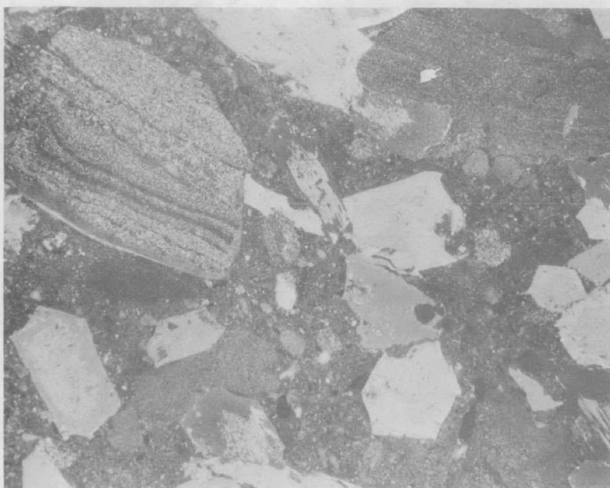
Fig. 14 Coarse euhedral gypsum crystals (white to light grey) and laminated dolomite fragments in very finely crystalline dolomite matrix. Thin Section 60-50-0274. Depth 150.54 m (493'11") Plane polarised light. 20X
