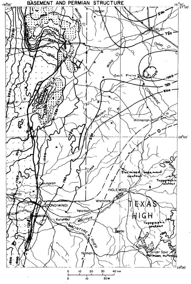
Fault Blackwater Group reflector Contour (metres below m.s.l.) on macament in B. Permian in W. Back Creek Group reflector (Lower Permian) Basement reflector, and Back Creek reflector basement from oil wells Eastern limit of U.K.A. saismic data and outerop information Oil well Southeastern limit of Phillips seismic data
