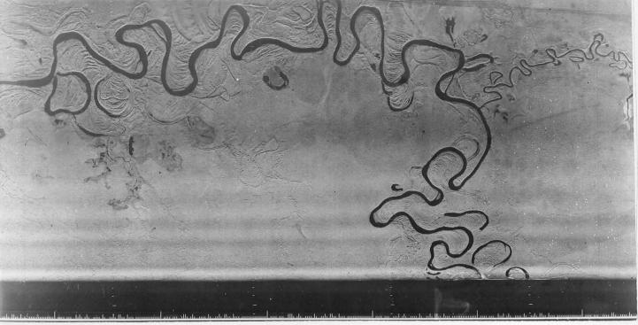
Fig. 1 SLAR imagery on adjacent runs. Note the variation in along-track (or azimuth) scale. This distortion was not expected in areas of low relief and low elevation.
