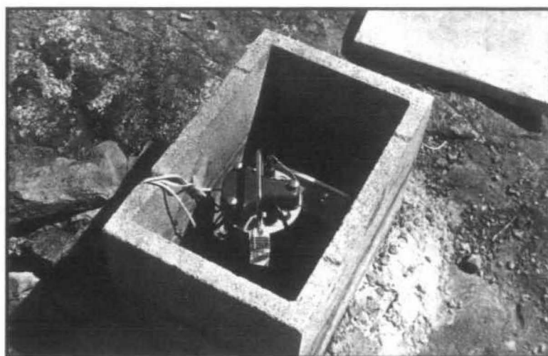
VAULT CONTAINING SEISMOMETER AND VOLTAGE AMPLIFIER
