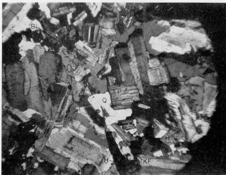
Plate 10, Figure 2. Hornblende-biotite microgranodiorite of the Maramuni Diorite in the lower Maramuni River. The rock consists of quartz(Q) and potash feldspar(KF) moulded on tabular crystals of plagioclase(P), with discrete crystals of hornblende(H) and biotite(Bi). x 35. (11NG1150).
