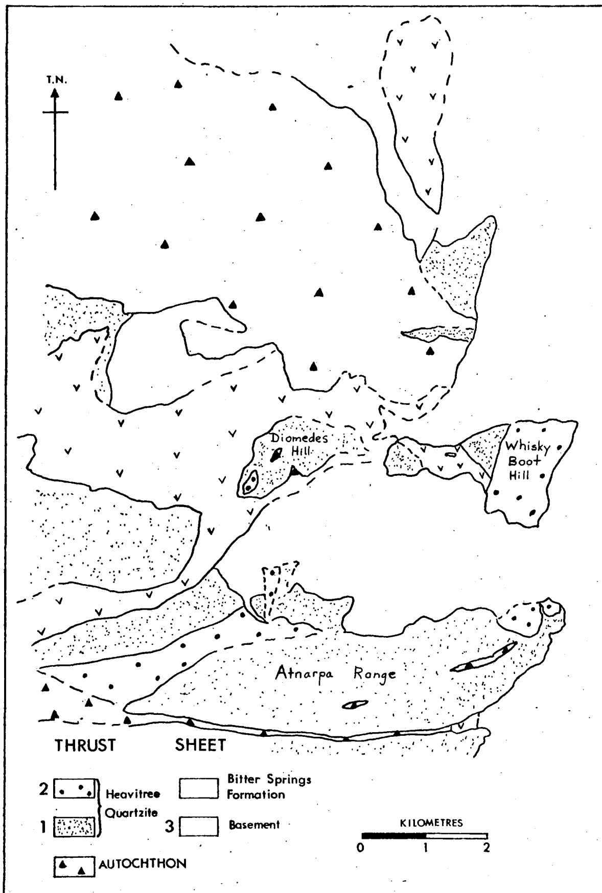
Figure 4 Structural level map of the Arltunga region. The thrust sheets are numbered in ascending order above the autochthon. To accompany Record 1973/10 F 53/A14/163
