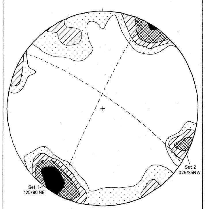
Poles to joint planes have been plotted on an equal area lower hemisphere projection and contoured to represent the distribution of joint directions. The orientations of joint sets are shown to the nearest 5 degrees. The curved clashed lines on the plot are the great circles which represent the joint planes.
