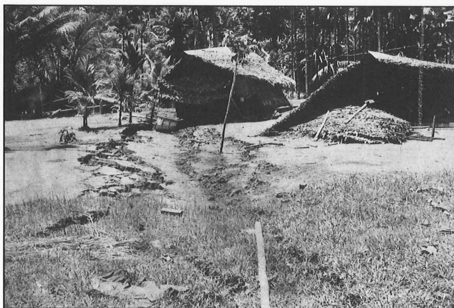
East-west tension feature. Length approximately 100 metres, caused by large scale slumping of ground parallel to river at left (outside picture). Near Sempri village.
