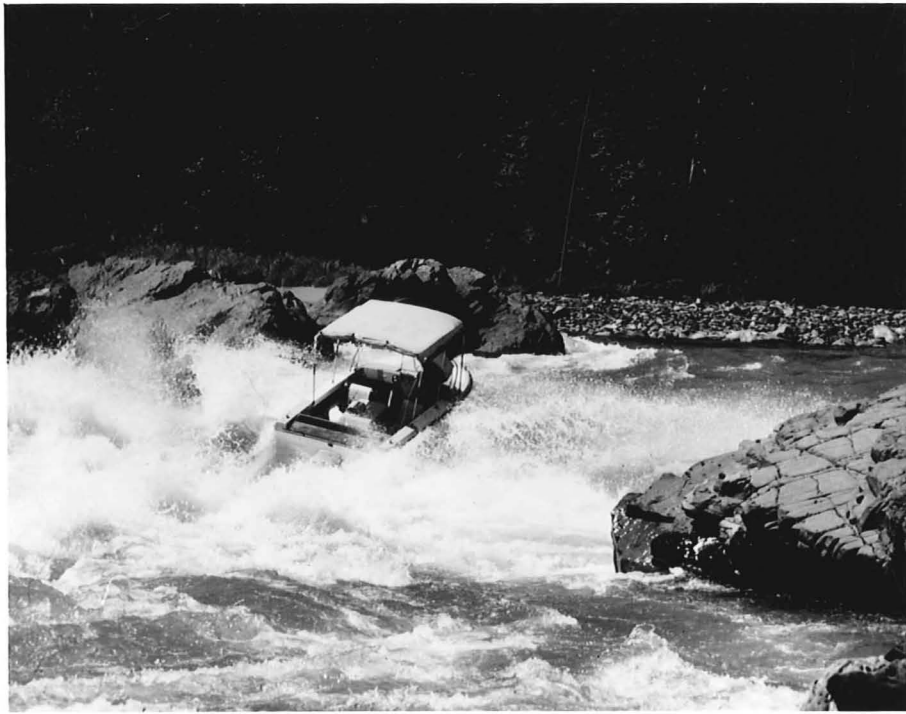
Figure 1: Jet-boat negotiating a difficult rapid in the Yuat River, South Sepik region. These boats, which can travel in as little as four inches of water penetrated the southern tributaries of the Sepik River well beyond the limits of conventional craft into the southern mountains.
