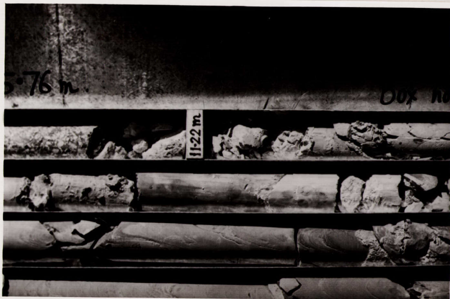
Photograph 9 (D52/4/115) Close-up of contact between conglomeratic sandstone and micaceous siltstone. Note complete weathering to a white clay, and other joints completely weathered to clay
