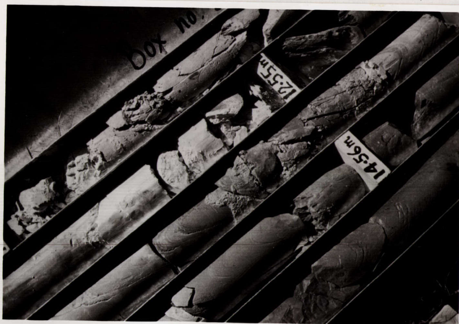
Photograph 10 (D52/4/116) Close-up of micaceous siltstone Note steep bedding and highly to completely weathered state of the siltstone
