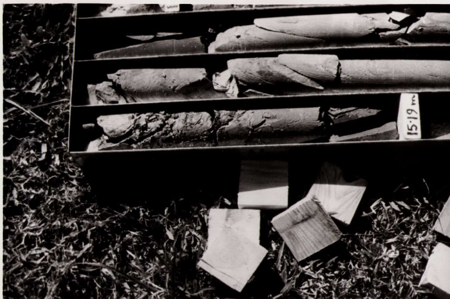
Photograph 11 (D52/4/117) Close-up of shear zone in highly weathered micaceous siltstone
