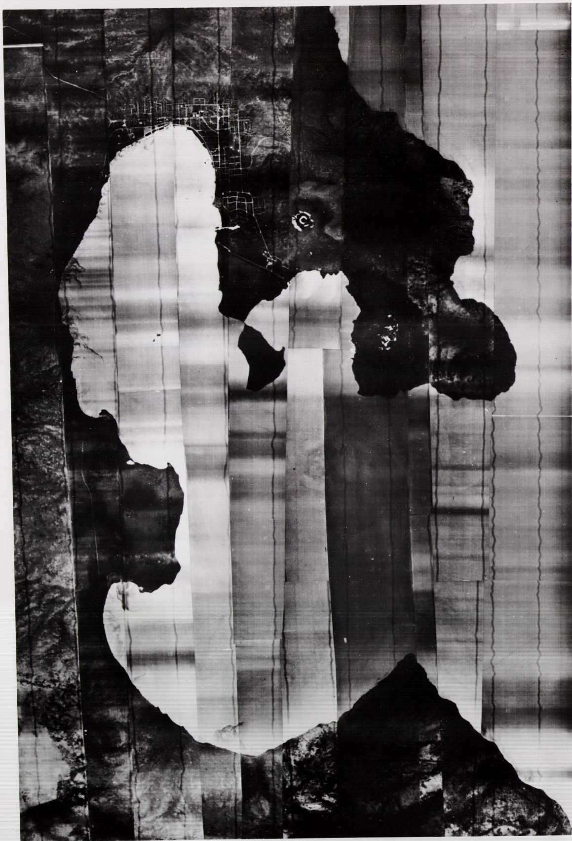
Fig 2 Mosaic of thermal infrared runs, 8-14 \mu m, Rabaul Caldera
