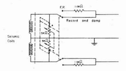
B. DAMPING AND F.P. CONTROL FOR MQI SITUATED IN VAULTLET
