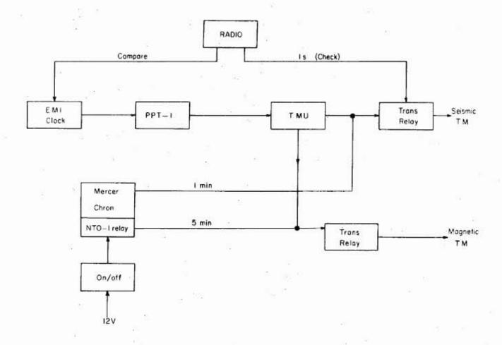
BLOCK DIAGRAM OF TIMING SYSTEM
