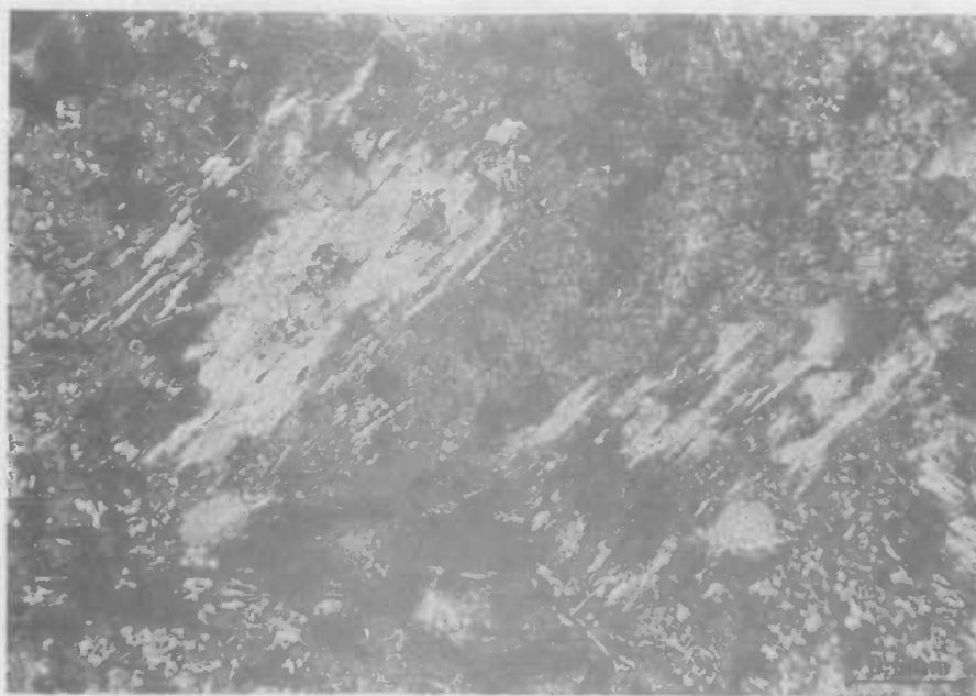
Fig. 7 - Photomicrograph showing ragged porphyroblasts of chlorite in gypsiferous dolomite rock. TS 71110295 from 283'1" (86.28 m). Crossed nicols.
