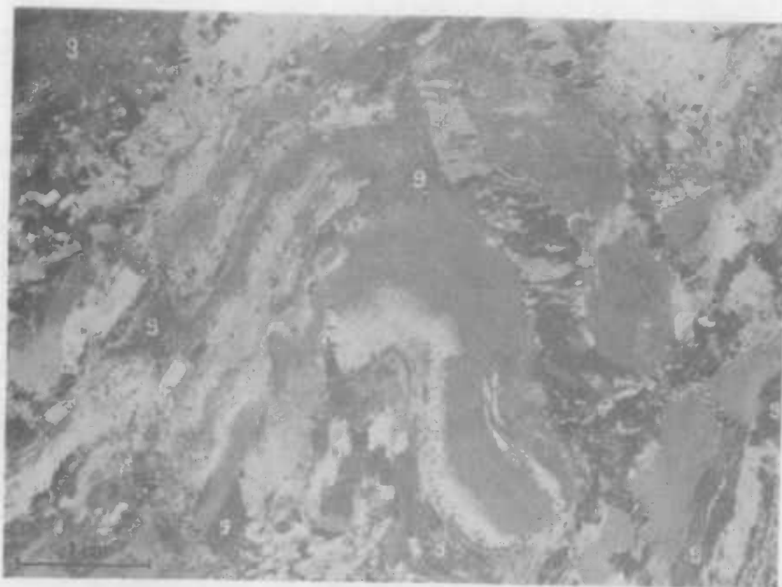
Fig. 14 - Photomicrograph of dolomite-gypsum breccia, showing contorted and broken laminae of gypsiferous dolomite rock in matrix of coarse poikilitic gypsum. Veins of prismatic to acicular gypsum may represent former solution channels, and grade into granular aggregates of stubby gypsum grains. g = gypsum poikiliths, in extinction position. TS 71110007 from 354'1" (107.92 m). Crossed nicols.
