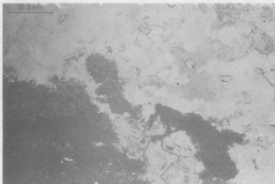
Fig. 13 - Photomicrograph of dolomite-gypsum breccia, showing ragged clasts of fine-grained gypsiferous dolomite and euhedral rhombs of recrystallized dolomite in coarse-grained granular gypsum. TS 71110001 from 116'10" (35.61 m). Plain light.
