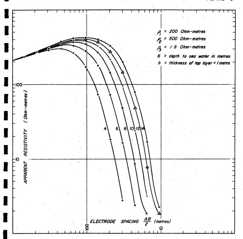
CHANGE IN SHAPE WITH DEPTH TO SEA WATER DURING PUMPING
