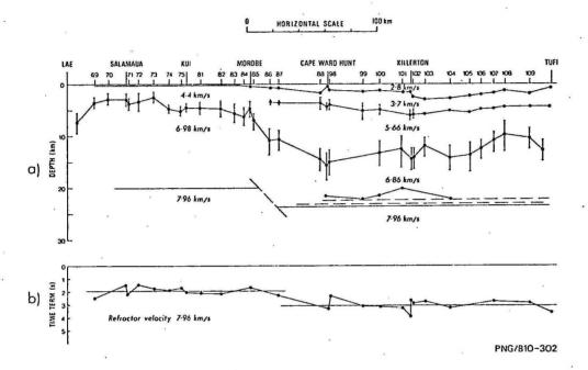
Fig.7 (a) Crustal structure along the Lae-Tufi profile.
