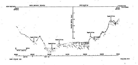
Fig.2 Seismic sparker traverse across the Solomon Sea from the Trobriand Platform to New Britain (location shown in Fig.3).
