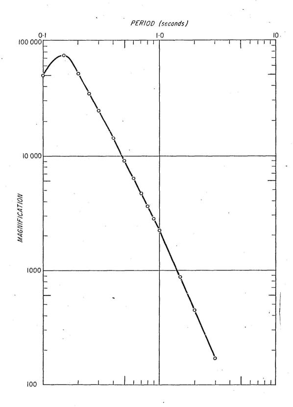
CALIBRATION CURVE TRANSPORTABLE SEISMOGRAPH
