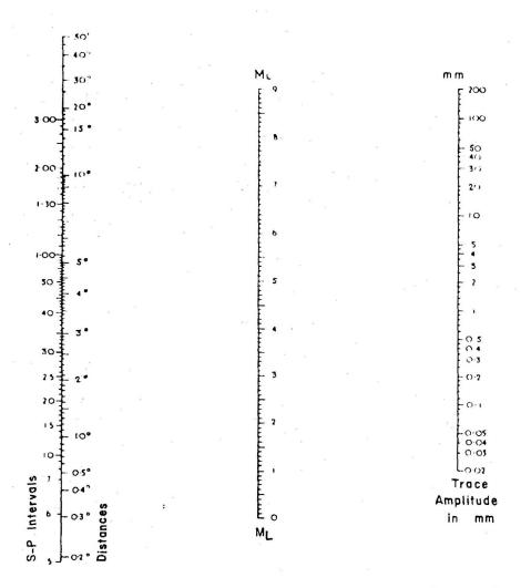
For use only with Wood-Anderson Torsion Seismographs having standard constants (Period O-8 sec, Magnification 2800, Damping h=0.8). The maximum trace amplitude is measured from the zero line. When two components are available use the arithmetic mean Corresponding values of distance, amplitude and magnitude lie on a straight line. S-P intervals shown are those for a focal depth of 0.00r.
