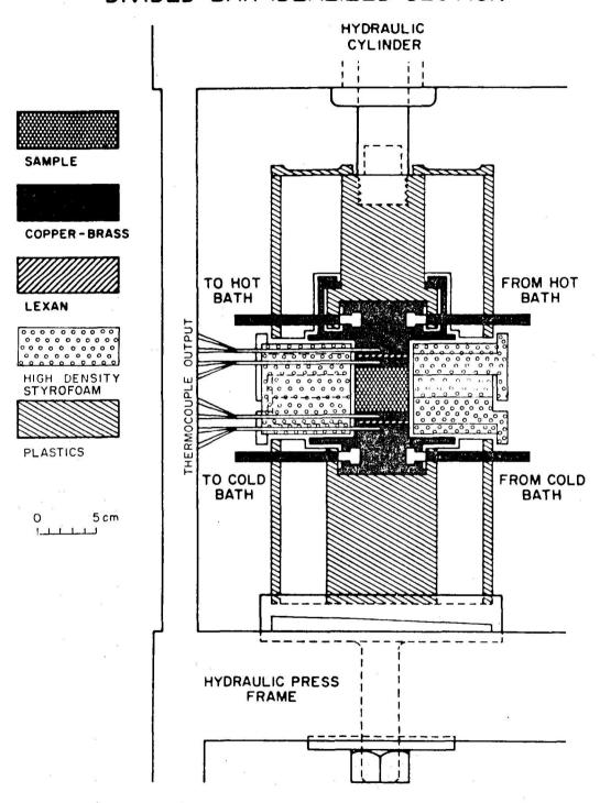
Fig. 6 Schematic diagram of divided bar apparatus for thermal conductivity measurements.
