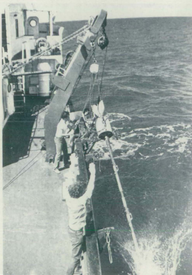
Fig.1B THE DROPPING OF THE CORE PIPE ABOARD RV VEMA
