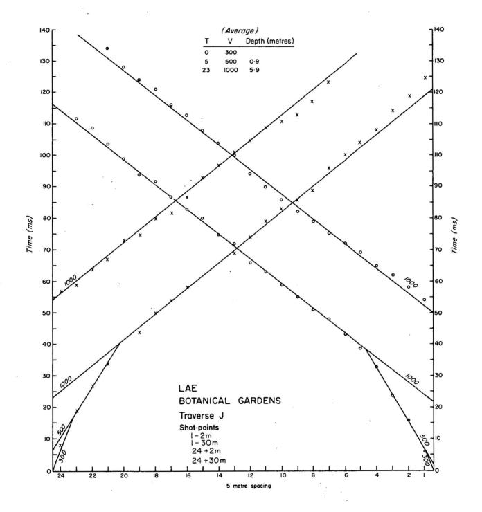
SEISMIC TRAVERSE J
