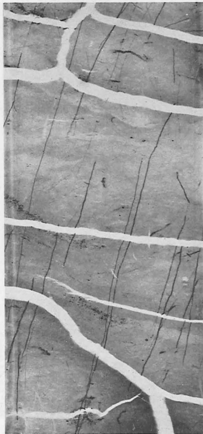
Figure 8. X-ray positive of thin vertical tubes in slice of Quaternary sediments in core BL 17 from the Java Trench. Depth in core = 40 cm to 60 cm. Natural size. White areas are desiccation cracks.
