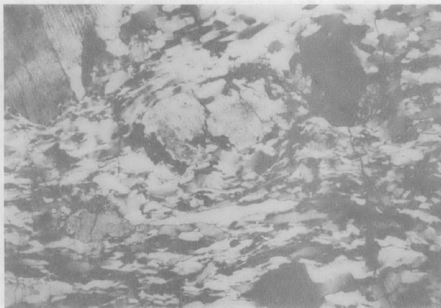
Figure 7b. Foliated augen granite, Bgs 1 , Waverley Creek area. Ovoid feldspar aggregates (clouded grains, centre of field and lower left of centre) are surrounded by ribbon-textured quartz. Crossed nicols, x 25.
