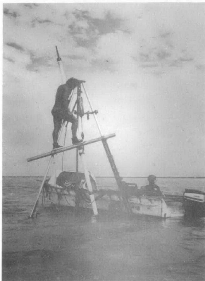
Fig. 9B Coring operations on the prograding sand sheet at One Tree. The core is 5 m long. The adapter connecting coring tubes to jackhammer is on top of the PVC tubes
