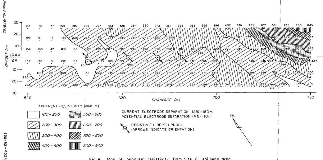
Map of apparent resistivity, Dam Site 2, spillway area.
