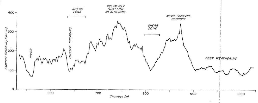
Fig.7 Dam Site 3. Resistivity profile
