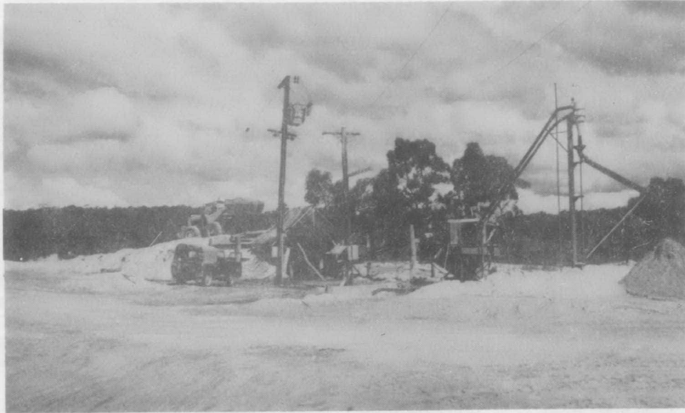
Figure 8. Washing of sand to remove fines at Deep Willows, near Braidwood (neg. no. M/2371/29)
