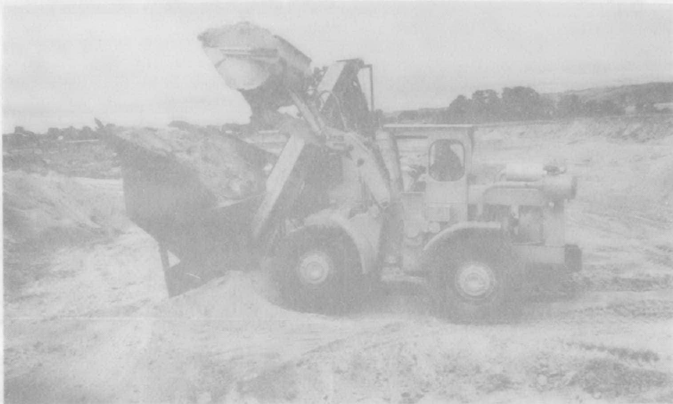
Figure 7. Dry screening of sand at the Canberra Washed Sands Pty Ltd Emersley, deposit, just north of Bungendore. (Neg. no. M/2371/28)
