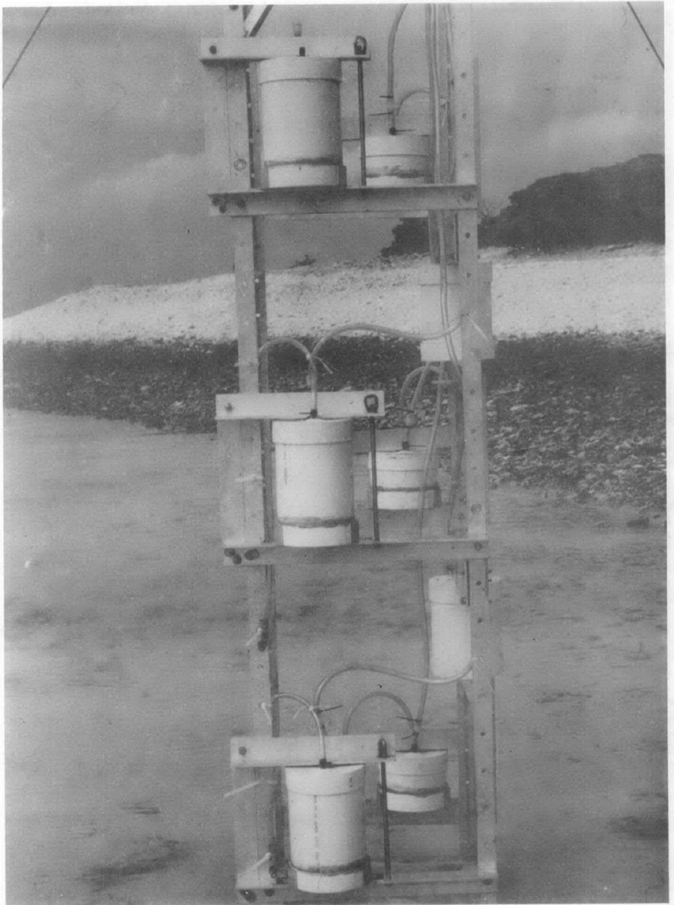
FIG 4-12-3 SEDIMENT SAMPLING TOWER
