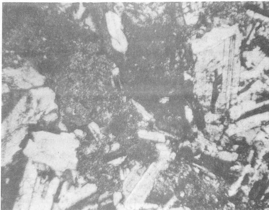
Fig 20: Photomicrograph of metadolerite showing well-preserved igneous texture (plagioclase laths); dark grey is hornblende. Specimen 75300033. Magnification X25 (crossed polars). Negative M2382/17.
