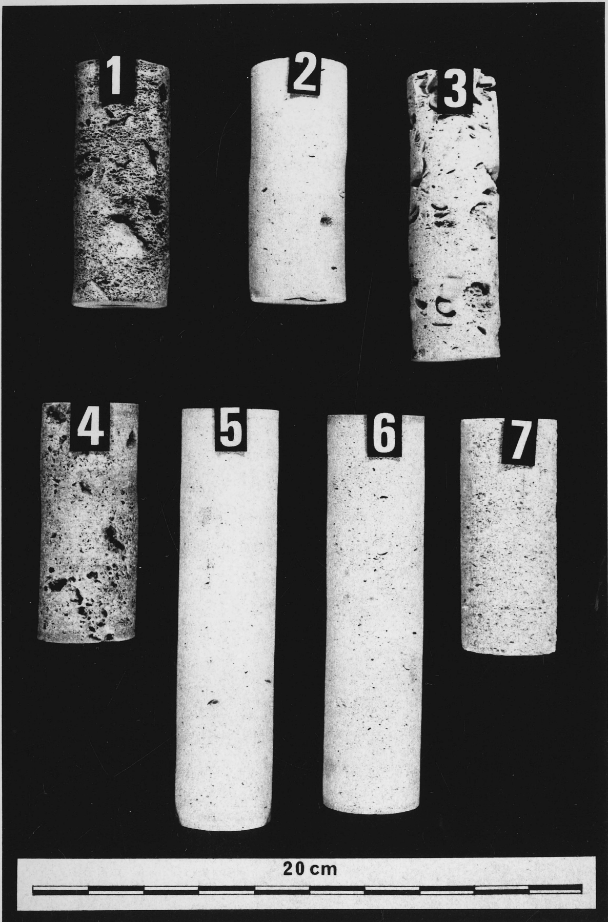
Fig.II. Typical core sections from the aquifer tested for resistivity and porosity (see text)
