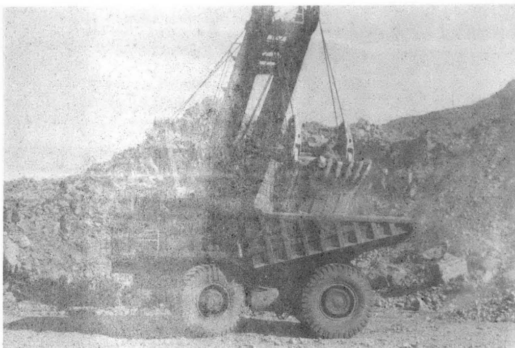
Fig. 31, Mining operations Dagushan pit WD 1200 12m 3 electric shovel loading Shaofeng 100t haulage truck. Both units are Chinese-built.
