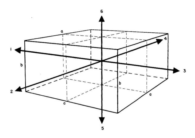
Fig. I Elemental volume of model based on square grid ax a for aquifer of thickness b, with six directions of flow
