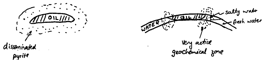
Figure 1.21 Geo-electric models of oil and gas fields showing regions of disseminated pyrite and associated IP anomaly.
