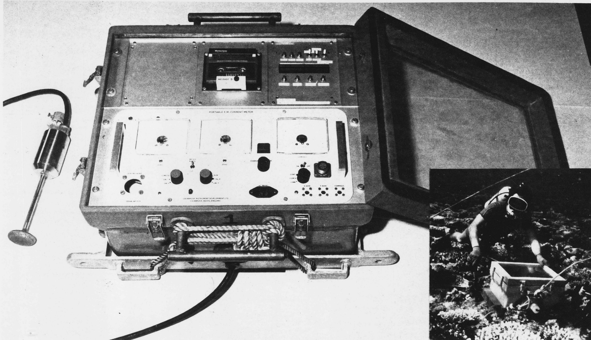
Fig 4.10.2 Borehole electromagnetic current flow meter for Great Barrier Reef survey. The equipment is housed in a pre-fabricated fibreglass container to withstand water depths of 10 meter. The microprocessor data acquisition system is in the upper part and the E.M. current sensor is on the left of the box.
