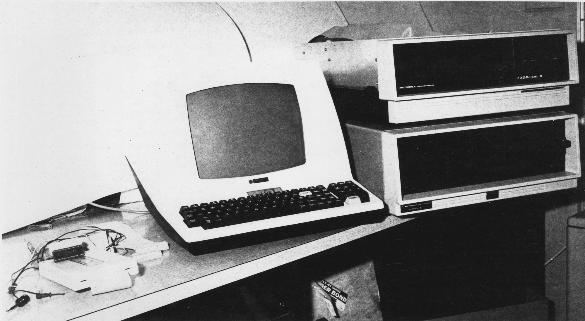
Fig. 4.12.3 The Exorciser II microprocessor development system provides a powerful tool for software development and hardware emulation, resulting in savings in development costs and time.
