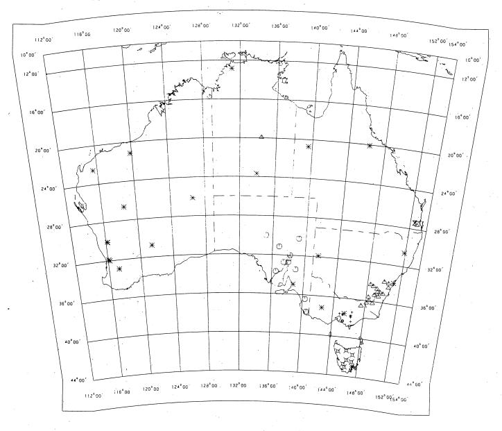
AUSTRALIAN NATIONAL SPHEROIS SIMPLE CONICAL PROJECTION WITH TWO STANDARD PARALLELS AT 18°00' AND 36°00' SOUTH
