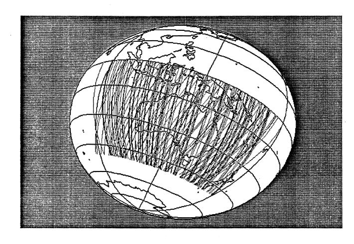
Figure 1 Geographic distribution of MAGSAT data held in the BMR MAGSAT\_DATA ORACLE database. The data comprise 163 passes of the satellite over the Australian region (0 to  $50^{\circ}$ S and 82.9 to  $180^{\circ}$ E).
