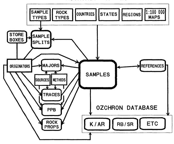
A schematic diagram of the PetChem database showing the main relationships between the PetChem tables. Also shown are some of the links with the OzChron database for geochronology results. Nearly all relationships are many to one, the arrow heads indicating the 'many' side of a relationship. The one exception is the link between SAMPLES and REFERENCES, where one reference may have many samples, but one sample can have up to 5 references.
