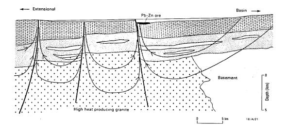
Figure 4. Possible stream lines during proposed ore-forming convection in basin sediments overlying a high heat producing granite.
