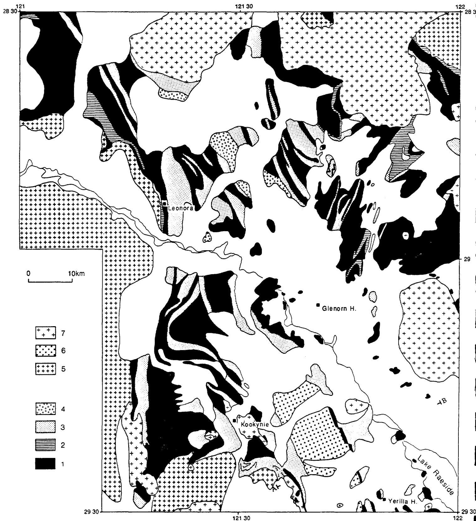
Figure 2. Simplified outcrop map of Archaean geology in the Leonora-Yerilla area. 1 - "Greenstone", comprising basalt, dolerite, gabbro, amphibolite, minor andesite. 2 - Ultramafic rocks. 3 - "Whitestone", sediments and rhyolitic to dacitic felsic volcanics. 4 - Polymict conglomerate. 5 - Granite-gneiss (pre- or syn-D1). 6 - Foliated granite (late D1 to syn-D2). 7 - Unfoliated granite (post-D2).
