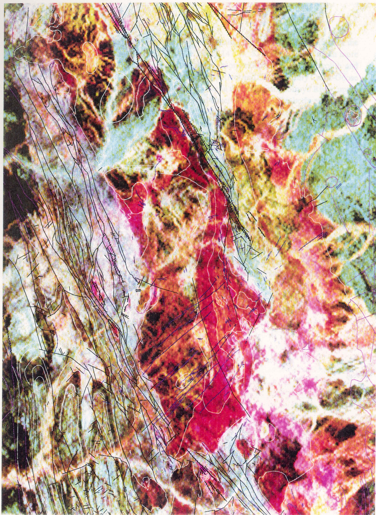
FIGURE 3. Pseudocolour gamma-ray spectrometric image of the Cape York Peninsula Batholith, EBAGoola showing geological boundaries (white), faults (black), and dykes (dark blue). Boundaries and faults in purple are from geophysics, as are most dykes.
