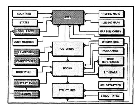
**Figure 2.** The structure of the NGMA Field Database showing relationships between tables with 'crows' feet' at the 'many' end of many-to-one links. The authority table labels emphasise function and are not necessarily actual table names (see below).
