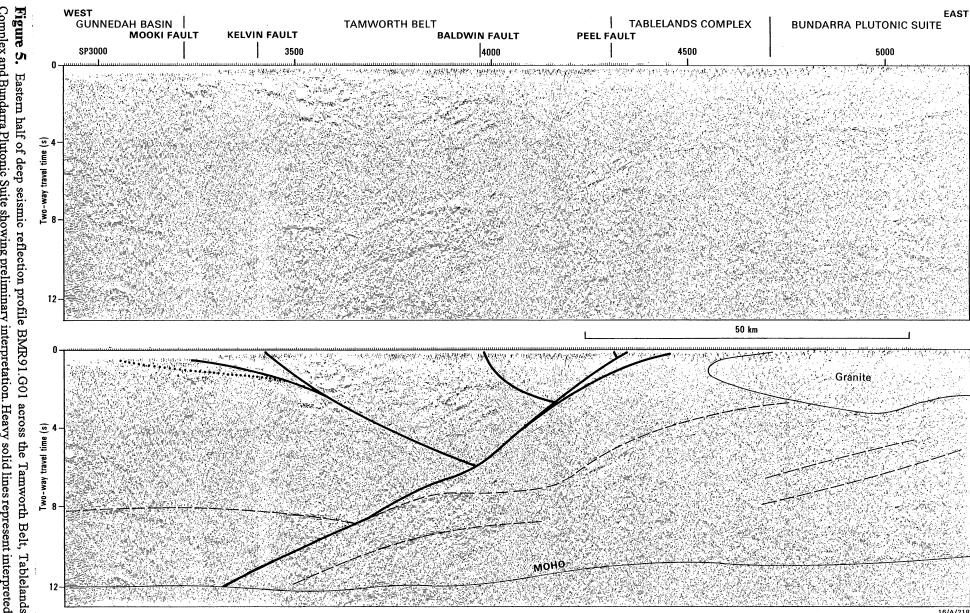
Complex and Bundarra Plutonic Suite showing preliminary interpretation. Heavy solid lines represent interpreted in upper right hand corner defines the shape of the Bundarra Plutonic Suite, and dashed units in the middle to lower crust. Note there is a slight amount of overlap with
