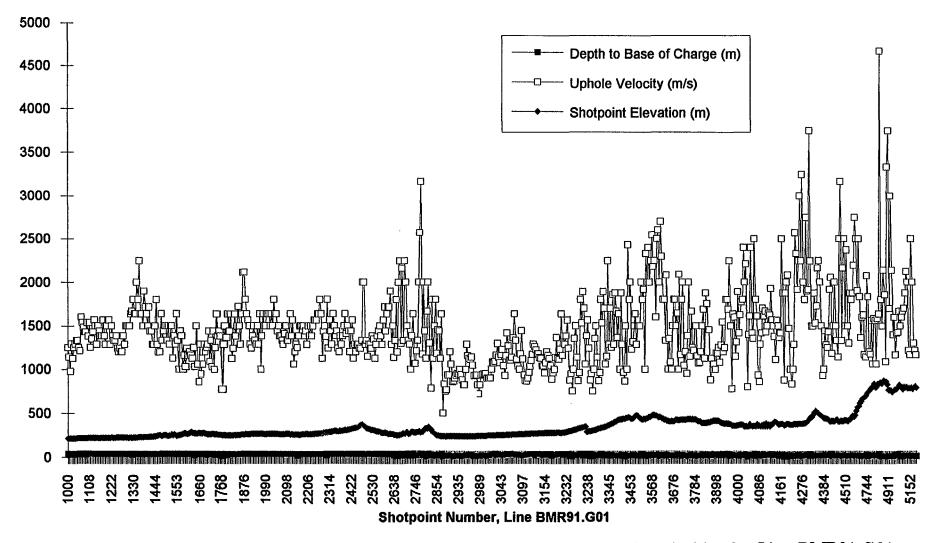
Figure 2. Shotpoint elevations, depth to base of charge and uphole velocities for Line BMR91.G01.
