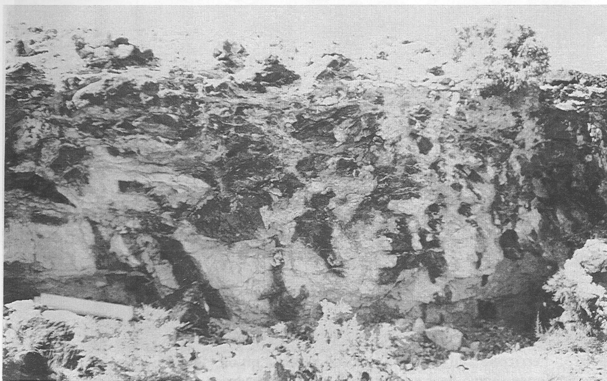
Figure 4. Ferruginous bedrock (mottles) within a weathered mafic granulite exposed in a pit wall on "Balaclava Station". (Scale 1: 50)
