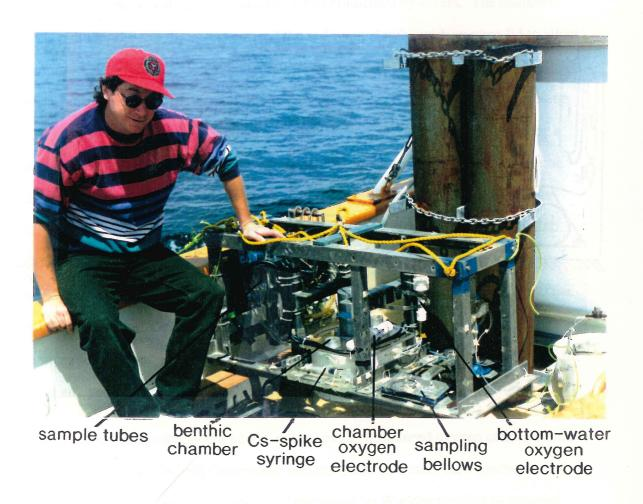
Figure 3. Photograph of the benthic chamber used in Port Phillip bay for these shallow-water deployments-key parts are highlighted.
