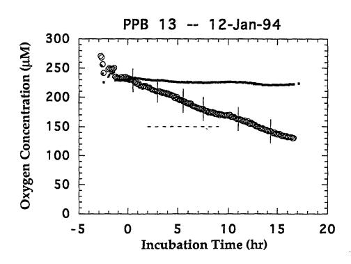
Figure 8. Oxygen concentration versus time from Sites 11 and 13 in the Central Zone of Port Phillip Bay.
