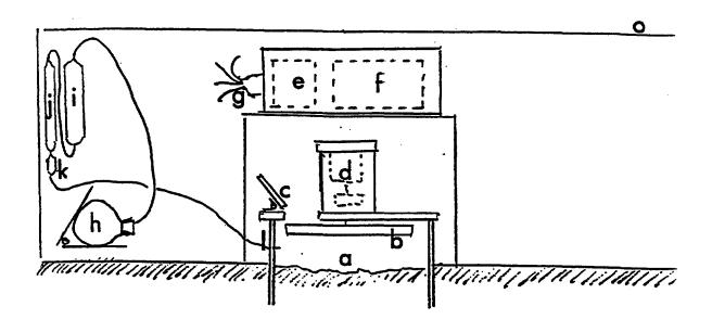
Figure 2. Schematic of the benthic chambers. Unit consists of a single cylindrical chamber (a), supported by an aluminium frame (o), that is approximately 1.2m x 0.5m x 0.5m. Other components include; chamber stirring paddle (b), hinged lid to top of chamber (c), pressure case with magnet-turning motor (d), pressure case with timing unit/micro-processor (e) and batteries (f) with burn wire leads (g), bulb that draws samples (h), sample tubes (i, j, k), tubing leading out of chamber (l).
