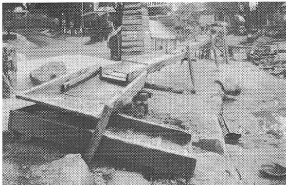
This slide shows a Broad Tom at the end of a sluice. The sluice is the long wooden channel which has a number of small pieces of timber, called riffles, on the bottom. The fine gold becomes trapped in these riffles in the same way that gold becomes trapped by slabs of rock in a creek. The Broad Tom is a section at the bottom of the sluice where miners could sort through the larger rocks and gravel, looking for nuggets and discarding everything else.
