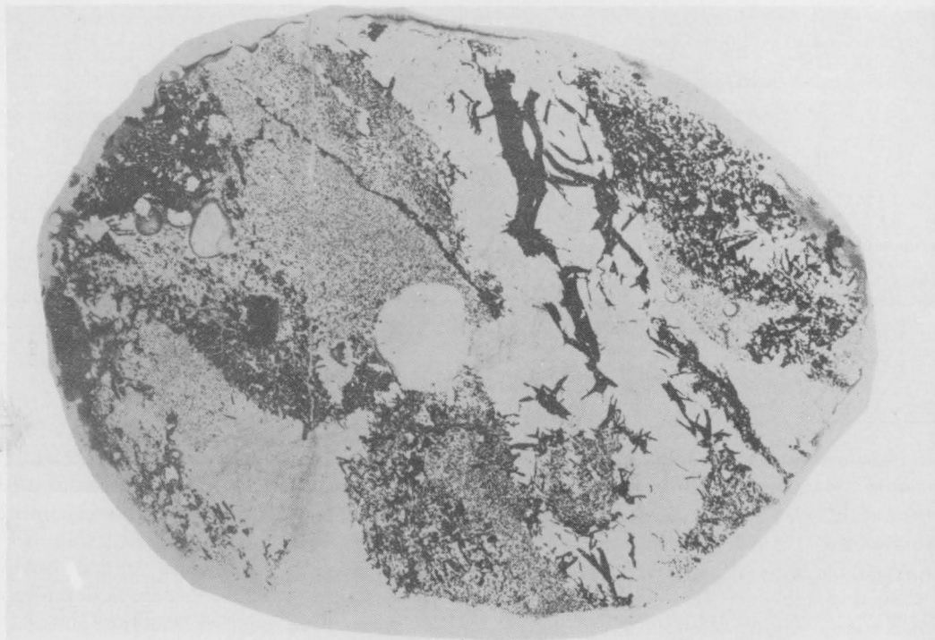
Fig.1 — Specimen A7193, showing deposition of iron governed by grain-size of quartz, and along fractures in later vein quartz. Crossed nicols, X13.
