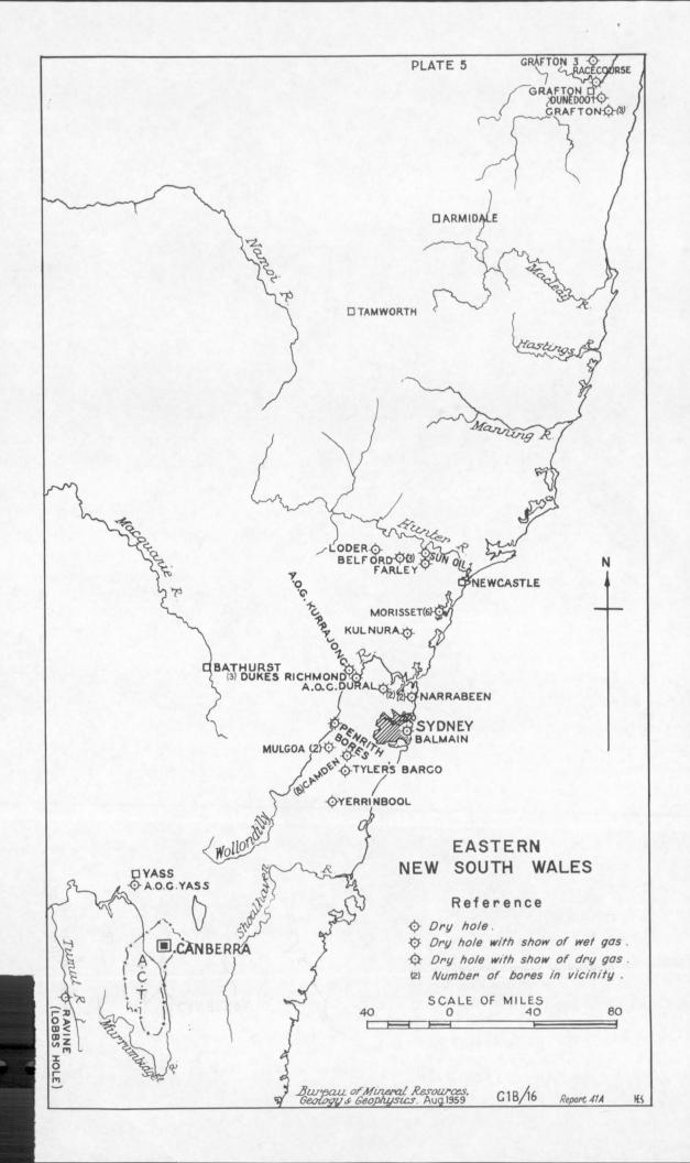
Farley Bore. This bore, drilled by W.J. Maskell, was suspended at a depth of 5,364 feet in 1936. The site was not well chosen: the bore started in steeply dipping sediments of the Permian Dalwood Group. Small gas shows were reported. A sum of about £12,000 was spent on drilling.
