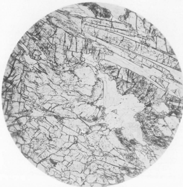
Fig. 2. Talc-tremolite-olivine rock (altered harzburgite) from Potai Creek, Fergusson Island. Pyroxene has been completely altered but olivine is quite fresh.
