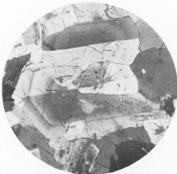
Fig. 1. Twinned and zoned plagioclase in the Omara Granodiorite, from near Wogawoga, Fergusson Island.
