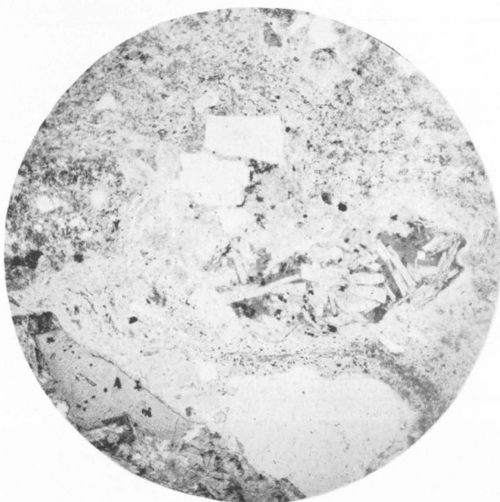
Fig.2. Devitrified ignimbrite showing phenocrysts of quartz and feldspar, one small rock fragment, and part of a large rock fragment. Edith River Volcanics, Mount Callanan Basin. Ordinary light, X35. Specimen R7668.
