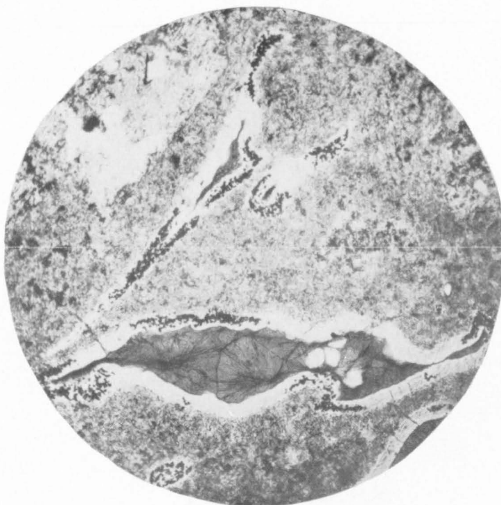
Fig.1. Devitrified ignimbrite showing former glass shards now replaced by fibrous, radiating chlorophaeite surrounded by a rim of quartz grains. The phenocryst is altered feldspar. Plum Tree Volcanic Member, Mount Callanan Basin. Ordinary light, X35. Specimen R7725.
