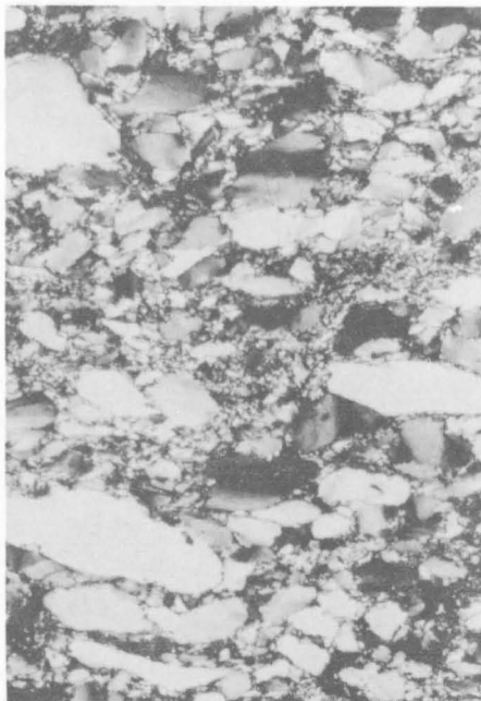
FIG. 2. Cataclastic quartzite. Specimen No. 65.660011. Crossed nicols, x 40.
