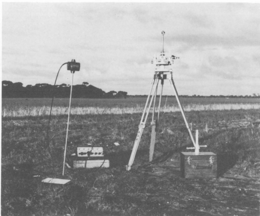
Elsec proton precession magnetometer, Askania declinometer and QHM magnetometer
